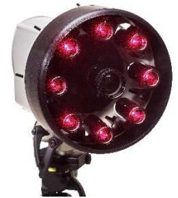
FlawExplorer sensor unit with 4 or 8 laser diodes for inspection of areas up to 2 m 2 (20 ft 2 ) in one shot
